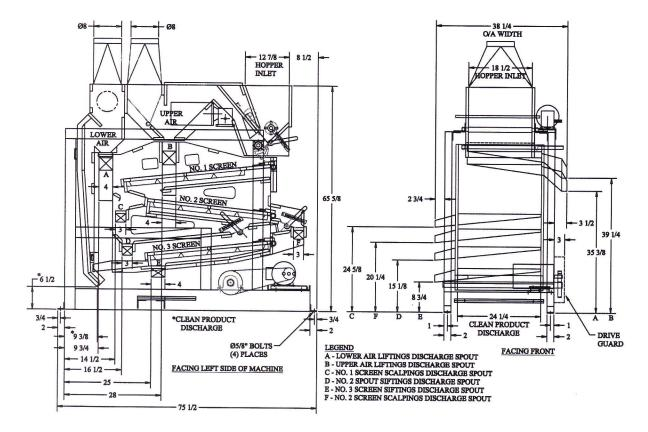
**The Crippen Micro 180** is designed for precision cleaning of small lots or low volume, continuous conditioning of seed. Quickly and easily cleaned out, controlled and flexible, the Micro 180 is adaptable to a wide variety of products and varying conditions.
